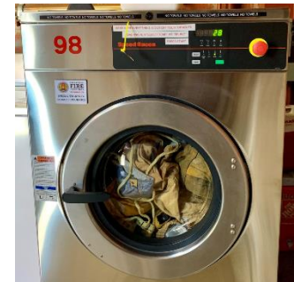
An extractor (above) purges toxins from turnout gear with the power and speed of 100-Gs (one hundred times the force of gravity).
