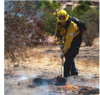
The rhino used by this firefighter is one of several specialized hand tools used to manually snuff out brush fires and hotspots.
